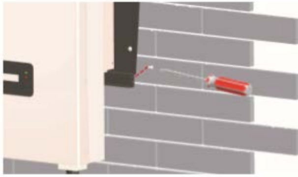
Figure 9 Fix the inverter
